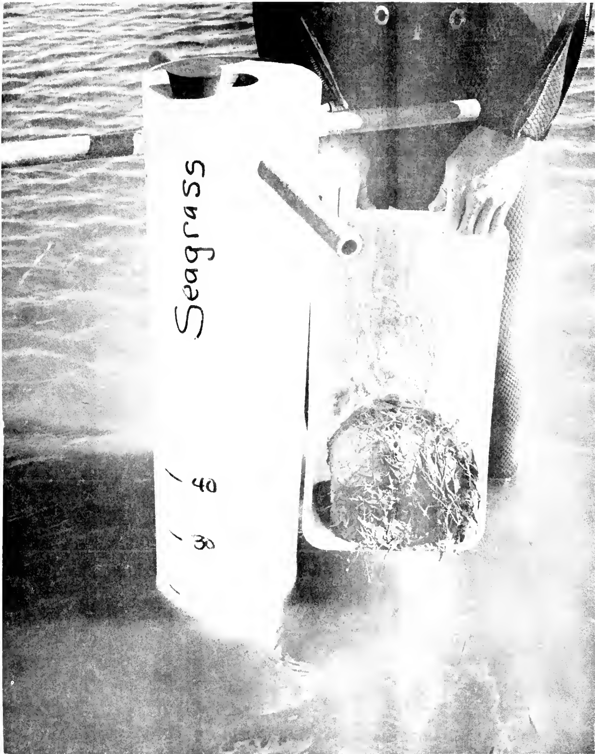
Figure 1. Coring device used for taking 20-cm (7.9-in) diameter plugs.
