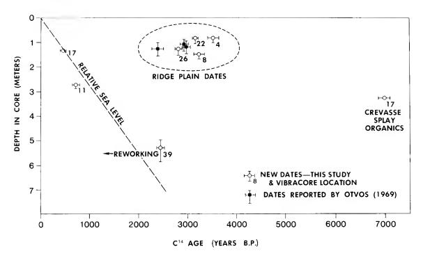
Figure 7. Inferred relative sea-level rise at the Caminada coast of Lafourche Parish (Gerdes 1982). The curve is based on radiocarbon-dated basal peats and in situ, articulated shells of <u>Crassostrea</u> <u>virginica</u>.
