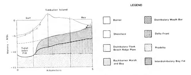
Figure 8. A stratigraphic strike section (top) and stratigraphic dip section (bottom) of the Timbalier Islands showing facies relationships and the infilled channel of Cat Island Pass offshore.
