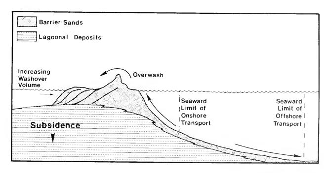
Figure 7. Two modes of coastal barrier sediment loss: (1) increasing washover storage, and (2) inequality in onshore-offshore sediment transport.
