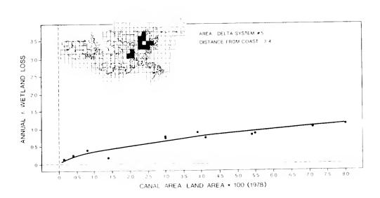
Figure 4. Land loss per 7 1/2'quandrangle for the delta system outlined in the map. Canal area is expressed as a percent of the total land area in 1978. This analysis and other examples are provided in detail in Scaife et al. (in press).
