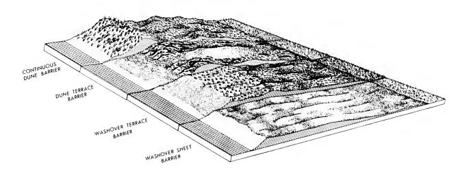
Figure 11. A three-dimensional landform diagram showing barrier types found in the Late Lafourche barrier system. Sediment availability for terrace and dune development decreases left to right, as does shoreline stability.
