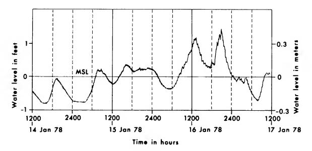
Figure 12. A tide gauge record segment from the western side of the Atchafalaya delta (Amerada Hess platform, Figure 3) showing the setup and setdown of bay water levels associated with cold-front passage (14-17 January 1978).
