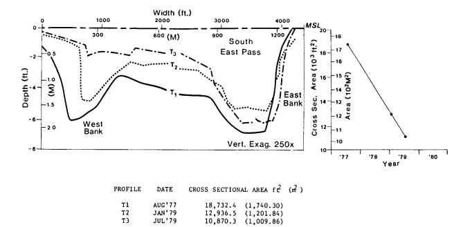
Figure 9. Profile of cross section in East Pass (see Figures 3 and 11 for location) showing the development of a mid-channel bar.
