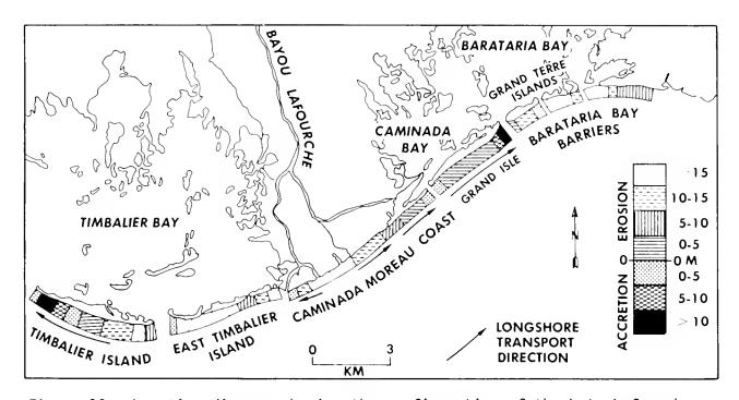
Figure 10. Location diagram showing the configuration of the Late Lafourche coastal barrier system and average rates of shoreline erosion and accretion.
