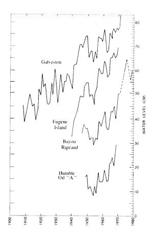
Figure 6. Yearly mean sea-level series for four stations along the north-central gulf coast. Data from tide gauges at Galveston, Eugene Island (at the entrance to Atchafalaya Bay), Bayou Rigaud (Grand Isle), and Humble Oil Platform "A" (13 km off Grand Isle). Data from Hicks and Crosby (1974) and Baumann (1980).
