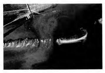
Figure 16. The ebb surge of Hurricane Flossy breached the Caminada Pass spit in 1956. Note the scour features along the shoreline formed by gulfward flow across the spit undergoing a hydraulic jump.
