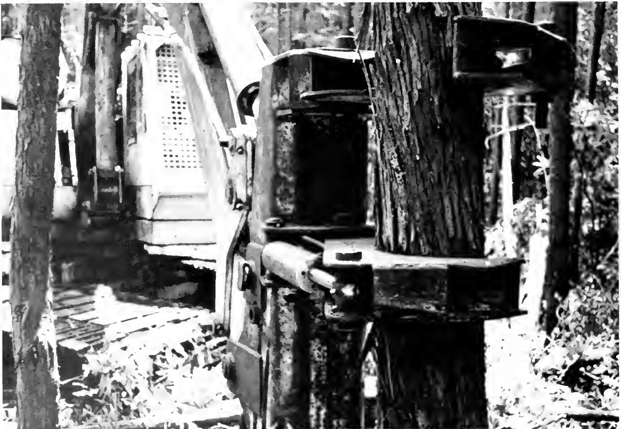
Figure 31. Amphibious feller-buncher harvesting Atlantic white cedar. Photograph courtesy Atlantic Forest Products, First Colony Farms, Edenton, NC.
