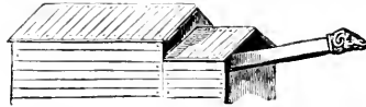
An aries , or battering-ram : from the Arch of Septimius Severus. The ram was a huge beam armed with a heavy metal ram's head. The ram represented is in a movable shed.
