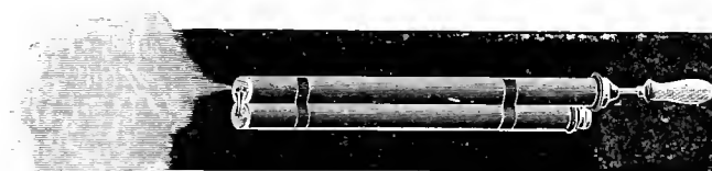
FIG. 16.—MR. C. E. WEST'S DOUBLE-BARRELLED SPRAYING SYRINGE, FOR EMPLOYING INSECTICIDES AND MIXING THEM WITH WATER.
