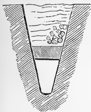
Fig. 14. Section of a Turf Drain.
