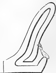
Fig. 55. Section of Mr. Saul's Pot.
