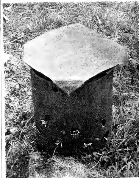
2.—A "NORBURY" HEATER WITH COVER ON READY FOR USE.
