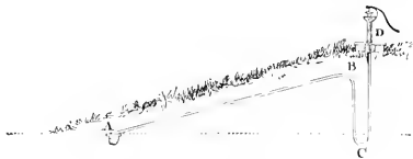
Pumping Water up a Slope.
