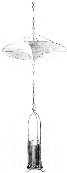
Lamp, for warming conservatories, &c., with cylinder and reflector.
