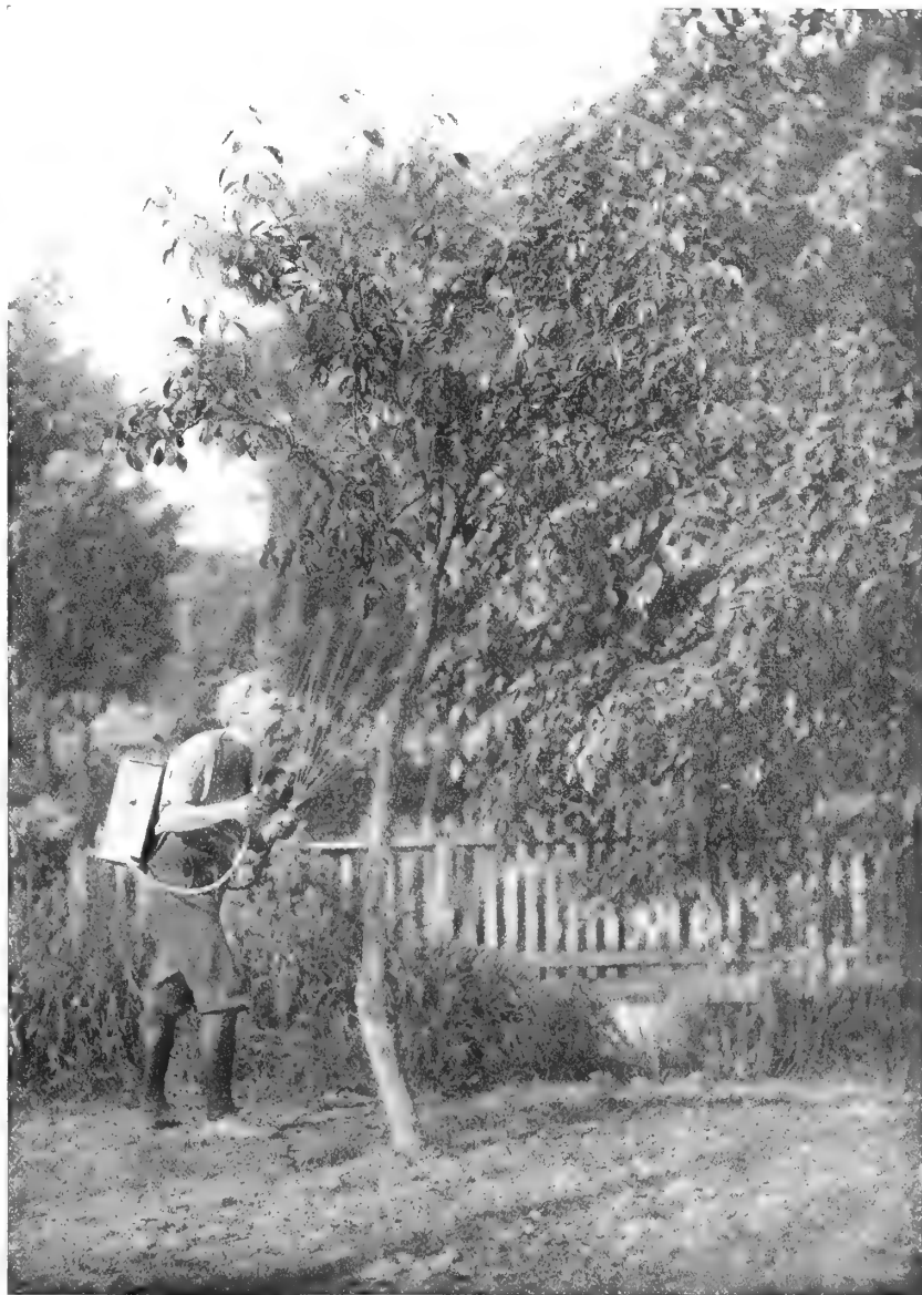
104. The knapsack sprayer in action. It weighs a ton after you have worked an hour in the hot sun, but it throws a spray fifteen feet high and is therefore useful for spraying trees as well as bushes and vegetables
