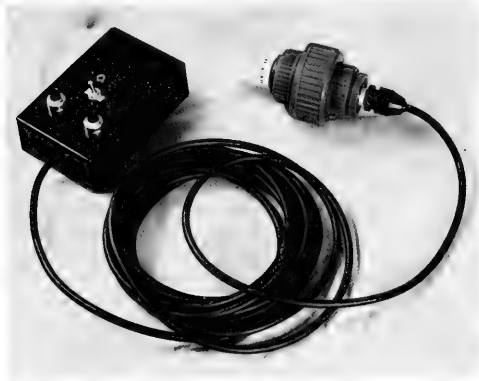
FIG. 1c Unit completed with approximately 30 ft of cable. R1 and R2 (see text) are on lower two corners of aluminum box; switch (S1) is in center below readout ( V_o ) jacks. Hair curler spool to hold silastic is shown without perforated metal protector.
