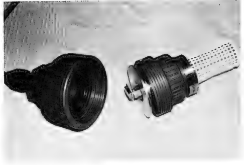
FIG. 1b PVC threaded pipe union which serves as submersible probe housing shown with brass insert containing Swagelock fitting in which pressure transducer (LX 1601AF) is mounted.
