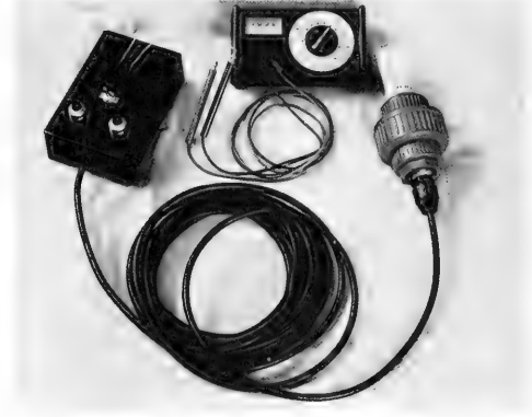
FIG. 1d Same as 1c but with digital VOM meter connected to output V_o .
