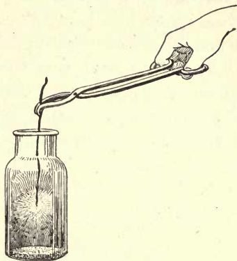
FIG. 84.—Burning Iron Wire in Oxygen.
