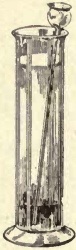
FIG. 44.—The copper sulphate solution slowly diffuses through the entire jar, as is shown by the change in color.
