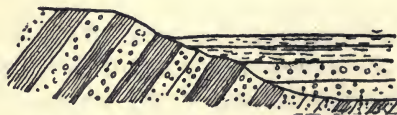
Fig. 20.—Diagram showing a Horizontal Series of Stratified Rocks laid on the Worn, Uptilted Edges of an Older Series
