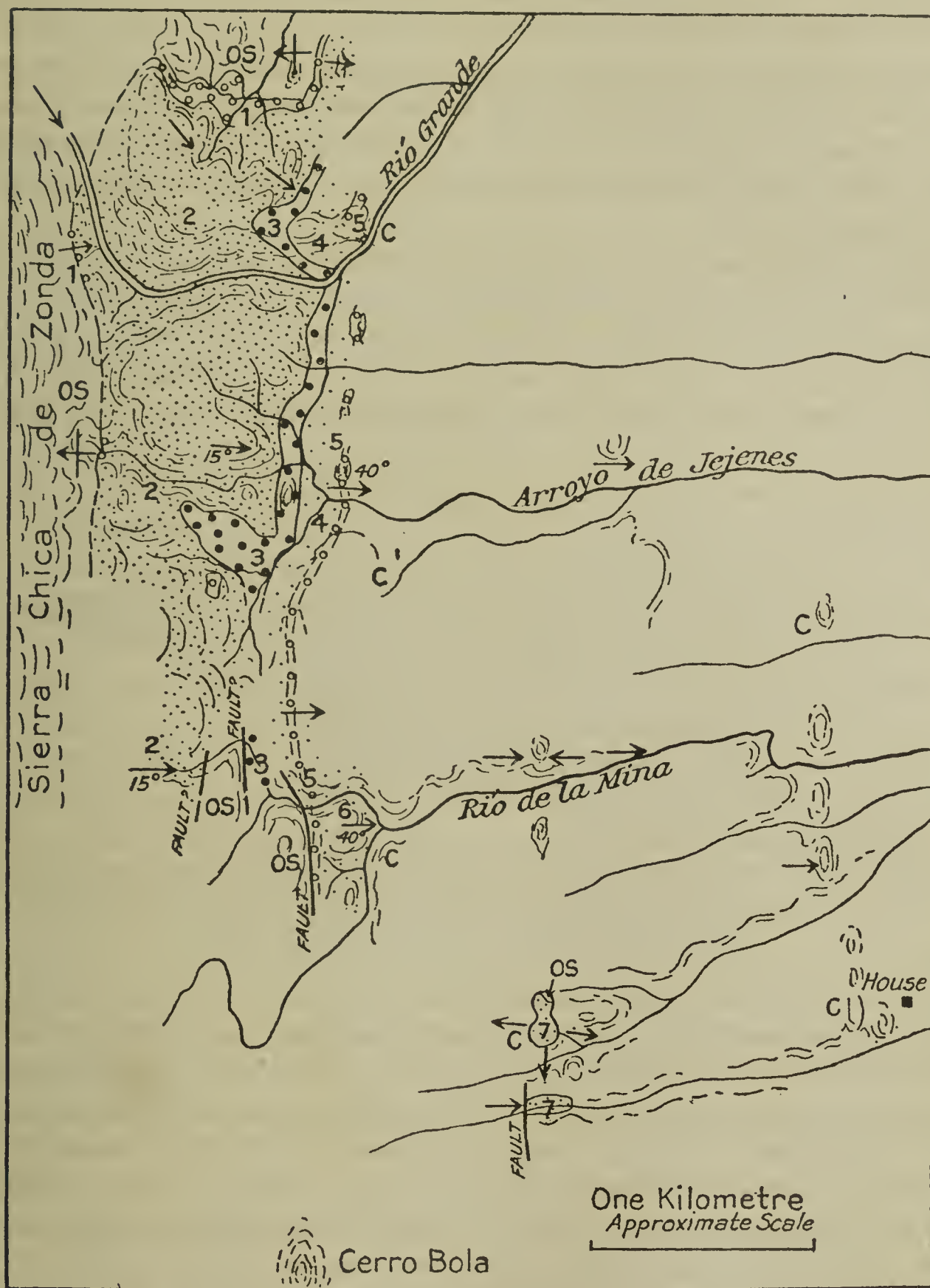
FIG. 2—Geological sketch-map of a small area along the eastern base of the Sierra Chica de Zonda to the south of San Juan. OS, Ordovician and Silurian limestones and shales. 1-7 Paganzo system: 1, first glacial zone; 2, plant-bearing shales and sandstones; 3, second glacial zone; 4, sandstones; 5, third glacial zone; 6, shales with some sandstones; 7, red and dark shales. C, Calchaqueños and Quaternary gravels.
