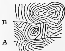
Concretionary Structure seen in old plastered wall, Co. Mayo, Ireland.
