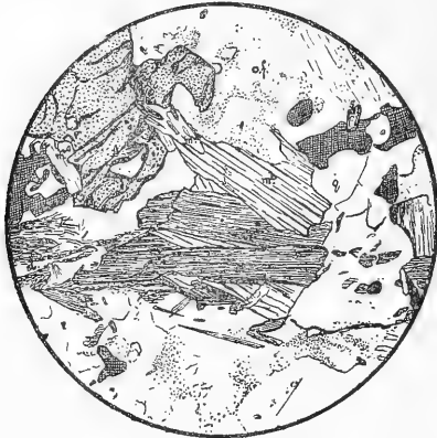
FIG. 1.—Usual type of the Darjiling gneiss, \times 20 . An irregular crystal of garnet appears on the left side towards the top of the stage. Near it are crystals of white mica ( m.w. ). The centre of the field is occupied by brown mica ( m.b. ); basal sections are cross-hatched. Sillimanite ( sl. ) is seen on the left side. The rest of the section is composed of orthoclase ( of. ), quartz ( q. ), and a single grain of sphen ( s. ).
