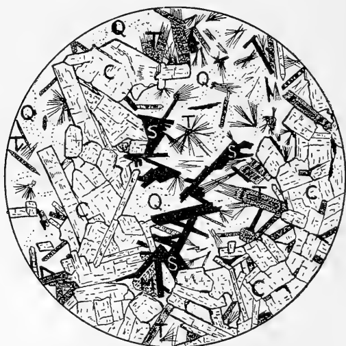
FIG. 3. Microphotograph of Specular Iron-Tinstone from Birch Tor. Q, quartz, all of one generation, in which the other minerals are set; C, cassiterite; S, specular iron; T, tourmaline; M, fine mica.
