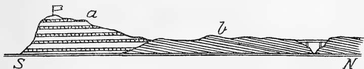
FIG. 2. Section Orewa Bridge to South Head. (a) Thin-bedded Tertiary sandstones and clays; (b) sandy clays with septaria.
