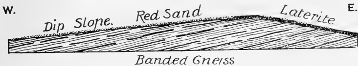
FIG. 1.—Typical Section in Maravi's country, north of the Mitikiti River, illustrating the occurrence of laterite on the escarpment slope of a ridge.
