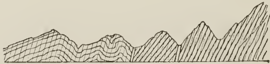
FIG. 64.—Figure showing slaty cleavage crossing, and also coinciding with the planes of bedding.
