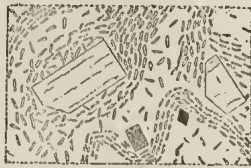
FIG. 14.—Microscopic section showing flow-structure of lath-shaped Felspars in Basalt.
