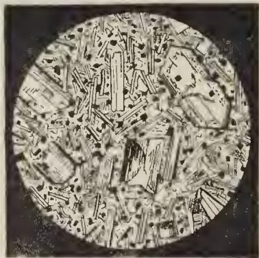
FIG. 8 —Microscopic structure of Basalt, Bald Hills, Bathurst.
