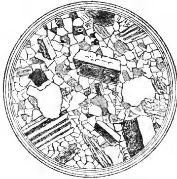
FIG. 17.—A thin slice of granite as seen under the microscope. The rectangular crystals are felspar, the clear mineral is quartz, and the shaded portions represent mica.
