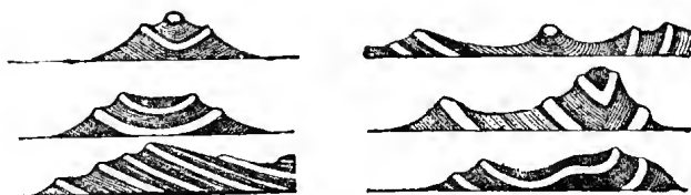
FIG. 83.—Diagram (after Dana) showing how the contour of hills depends on the unequal weathering of harder and softer rocks by denudation.
