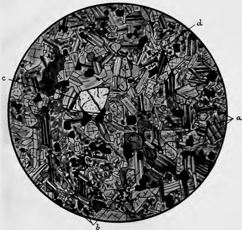
Thin Section of Basalt \times 75 (crossed Nicols). a , Augite; b , Felspar; c , Olivine; d , Decomposed Felspar and Glass.
