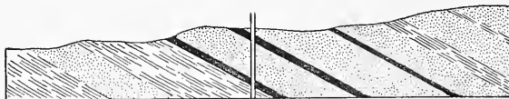
FIG. 29.—Case where a boring is the most economical and certain method of determining the presence of a series of coal beds in a given thickness of coal measures.
