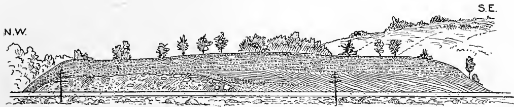
FIG. 33.—Section of terminal moraine covered by high-level flood gravels of the Westfield River. The north slope is caused by caving from the erosion of the river. Russell, just below station.
