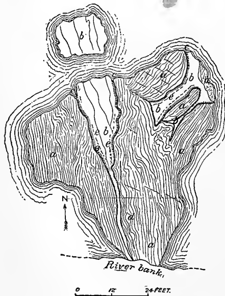
FIG. 6.—Map of emery veins in epidote-amphibolite at north end of bed on the bank of the Westfield River, Chester. a , Epidote-amphibolite; b , magnetite-emery beds; c , biotite fringe rock; d , quartz veins; e , tourmaline.
