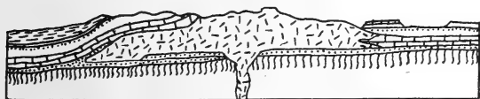
FIG. 325. — Diagram of a laccolith, showing the relation of the igneous intrusion to the overlying and underlying strata.
