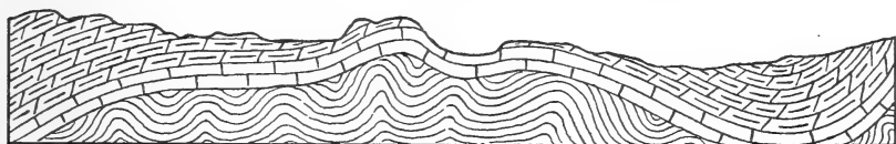
FIG. 394. — An east-west section in eastern New York, showing the Silurian resting unconformably upon the upturned edges of the Ordovician. (After W. J. Miller.) We have here the proof that this portion of the continent was raised above the sea during the Ordovician, and that after the land was eroded it sank, and upon this old land surface Silurian sediments were deposited.
