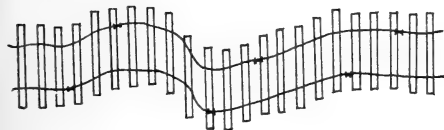
FIG. 284.—Diagram showing a railroad track bent during the Charleston earthquake.
