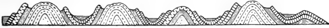
FIG. 344. — Section through the Juras, showing mountain ridges produced by several open folds, like great earth waves.
