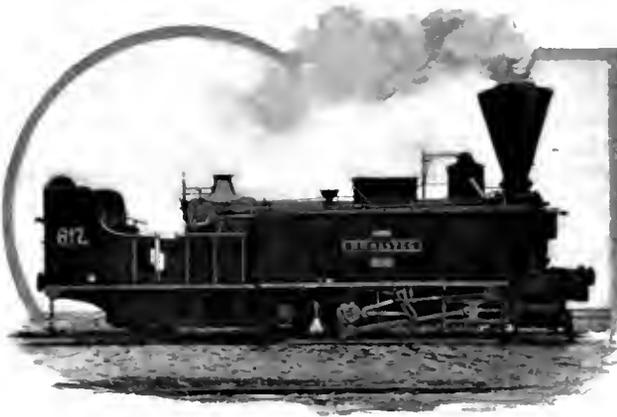
Abb. 267. Locomotive System Engerth. [Kessler 1853.]
