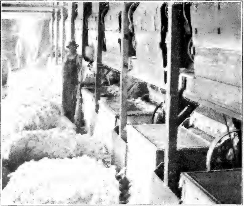
FIG. 1.—A 10-STAND GIN WITH FLAPPER-ROLLER ATTACHMENTS FOR REMOVING THE LINT FROM THE ROLLER
