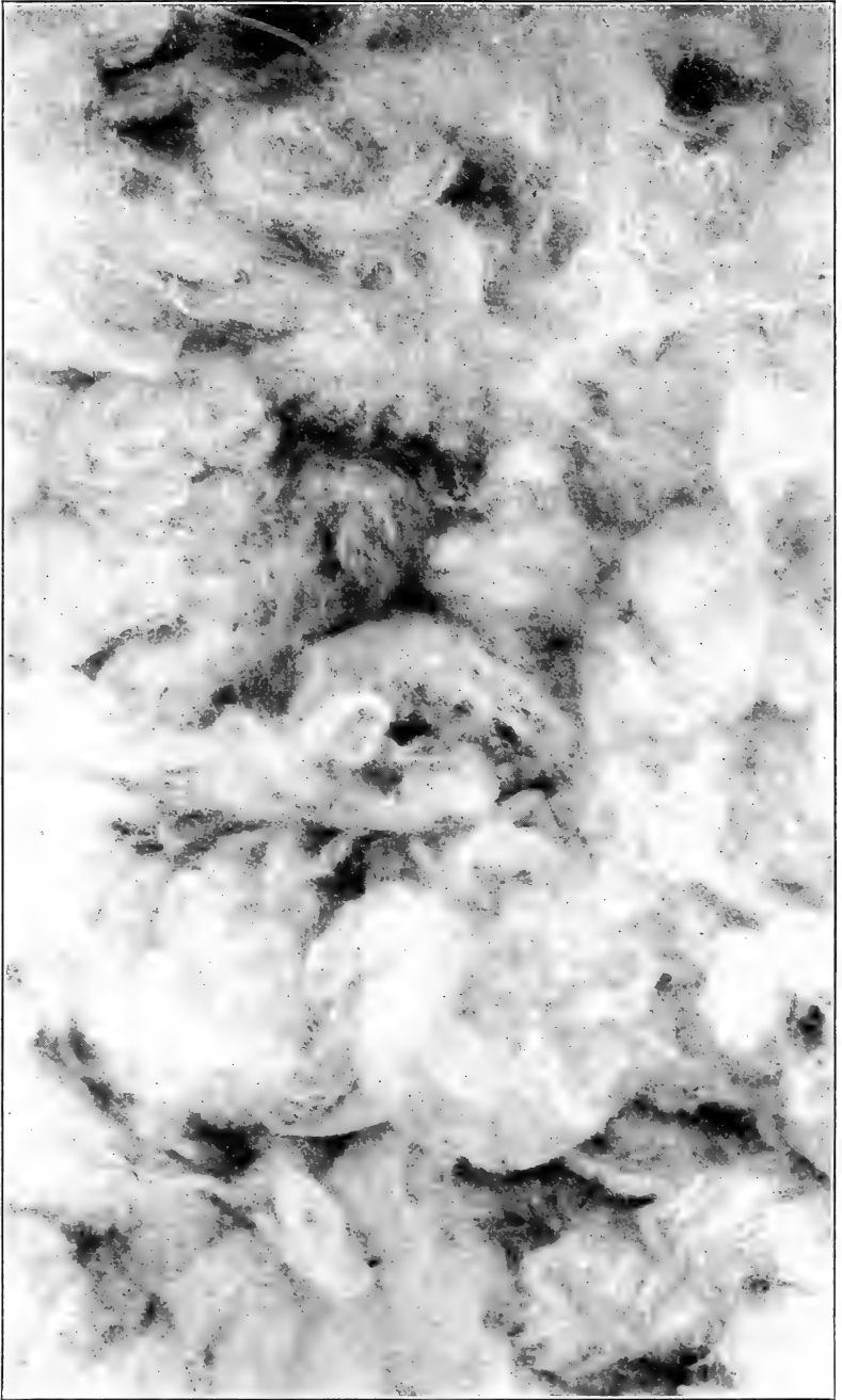
SAMPLE OF LINT AFTER IT HAS BEEN IN CONTACT WITH THE BRUSH Note the curled and rough appearance in comparison with the lint shown in Plate XI
