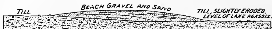
FIG. 6.—Typical section across a beach ridge of Lake Agassiz. Scale, 100 feet to an inch.
