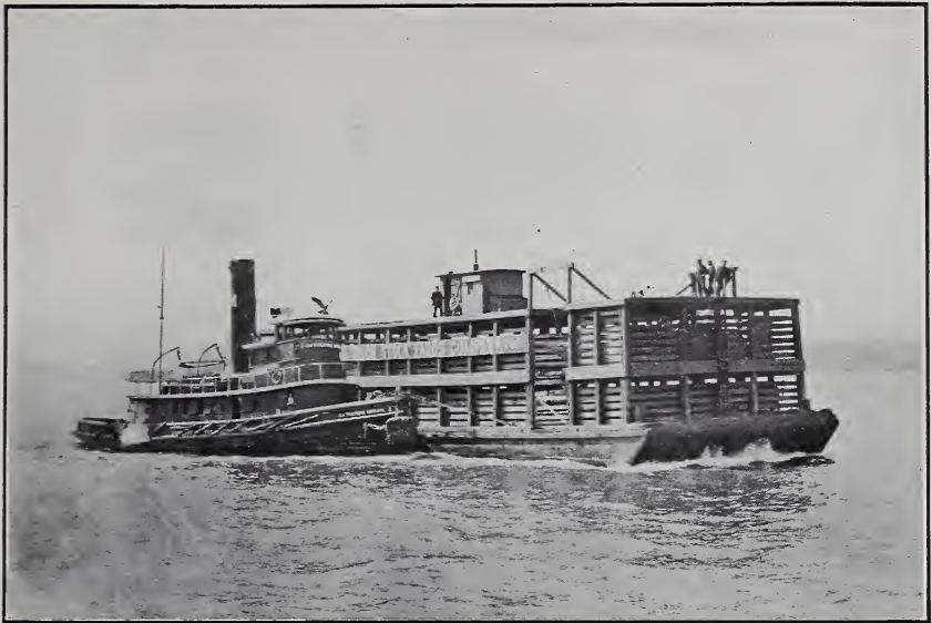
FIG. 1.—LIGHTER CARRYING EXPORT CATTLE FROM JERSEY CITY TO STEAMER DOCK IN NEW YORK HARBOR.
