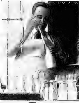
No. 1. Drawing sample (17.5 c.c.)
