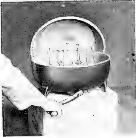
No. 4. Whirling in Babcock Tester (5 min.)
