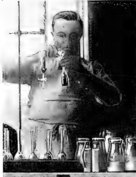
No. 5. Adding hot water (It is then whirled another min.)
