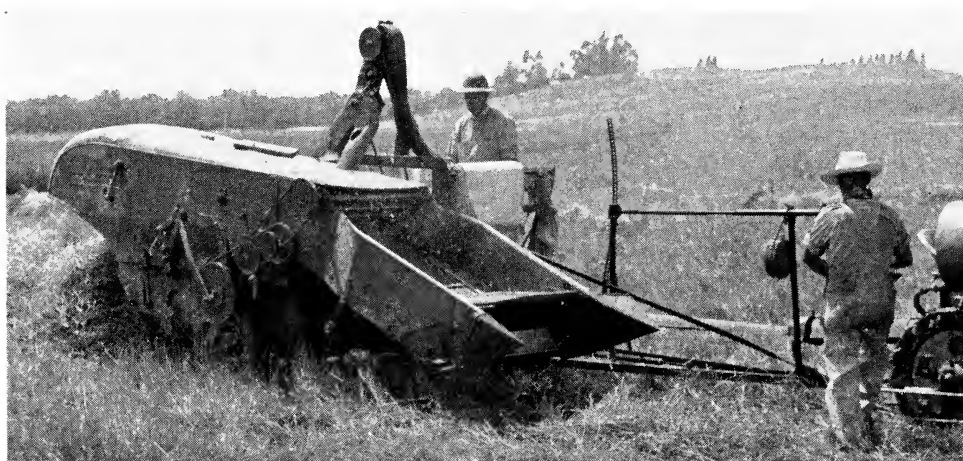
Fig. 8—Standard combines can be used as mobile threshers moving from one group of shocks to the next. The cut bundles should be evenly spread over the draper to provide an even flow of material into the thresher.
