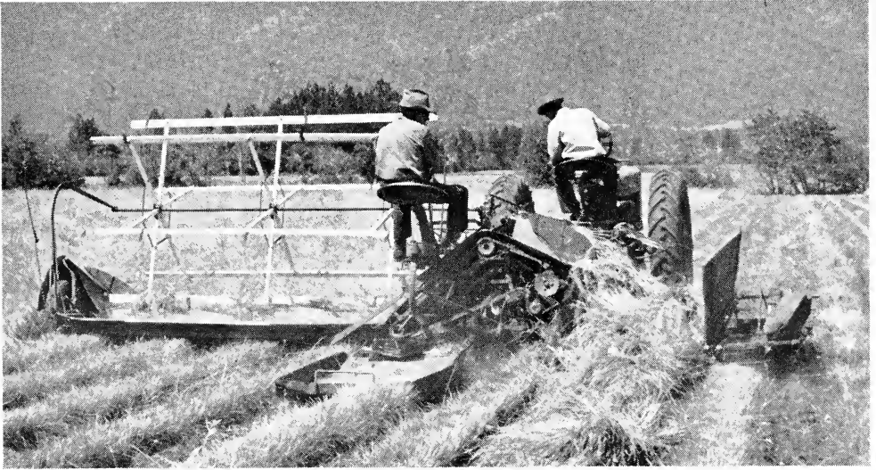
Fig. 5—Binding, shocking to cure and threshing with a mobile machine is the most widely used grass seed harvesting method. The shattered seed on the left of the machine sifts into the metal pan shown dragging beneath and extending to the rear of the binder. Shattered seed from the right side of the machine slides into the tray beneath the bundle carrier. Note short pieces of hose fastened to reel slats. These are centered on the rows and help to keep the cutter-bar free. (Union Pacific Railroad photo.)
