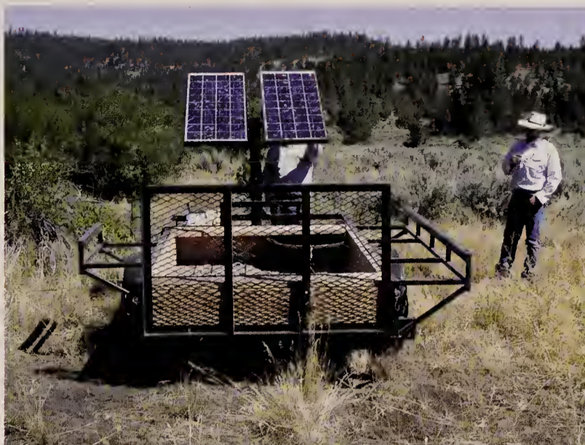
Figure 20. Mobile solar powered pump.
