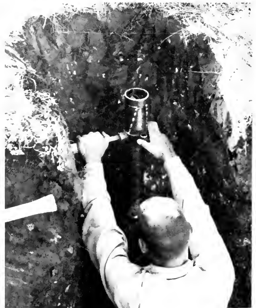
Fig. 2. Root samples were obtained using a core sampler driven into the soil to a 122-cm depth by 15-cm increments.
