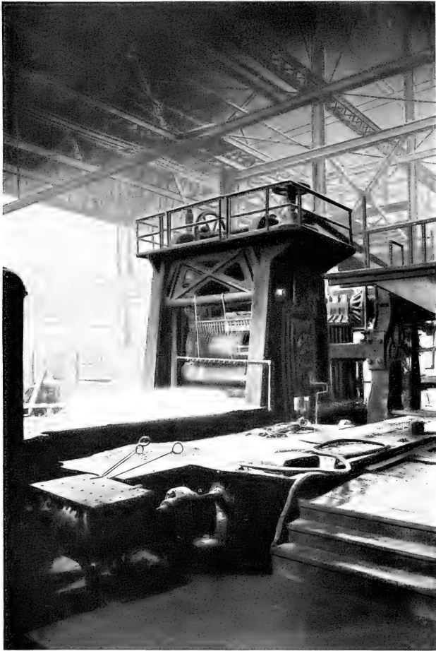
White-hot steel ingot being rolled in the slabbing mill. Courtesy of the United States Steel Corporation
