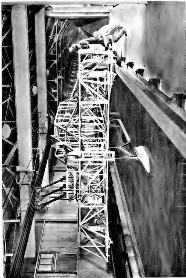
N.A.C.A. scaplane channel. Interior view showing towing carriage and float model in position. Courtesy of the National Advisory Committee for Aeronautics
