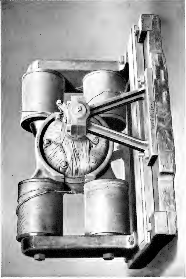
Original Thomson three-phase dynamo. Wound by Dr. Elihu Thomson in 1879. In the National Museum
