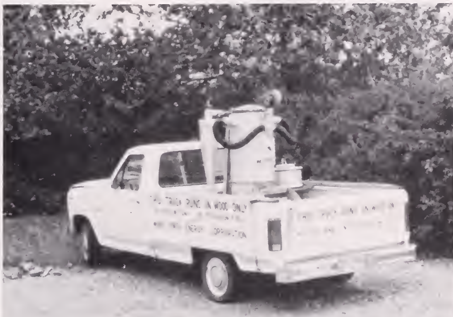
This truck runs on wood. The large tank behind the cab converts wood chips to gas. One dead limb will take the truck 100 miles.
