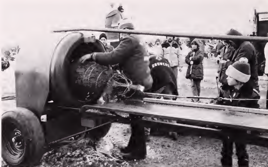
A quick trip through the baling machine makes the Christmas trees much easier to stow in the car and get in through the doorway at home.
