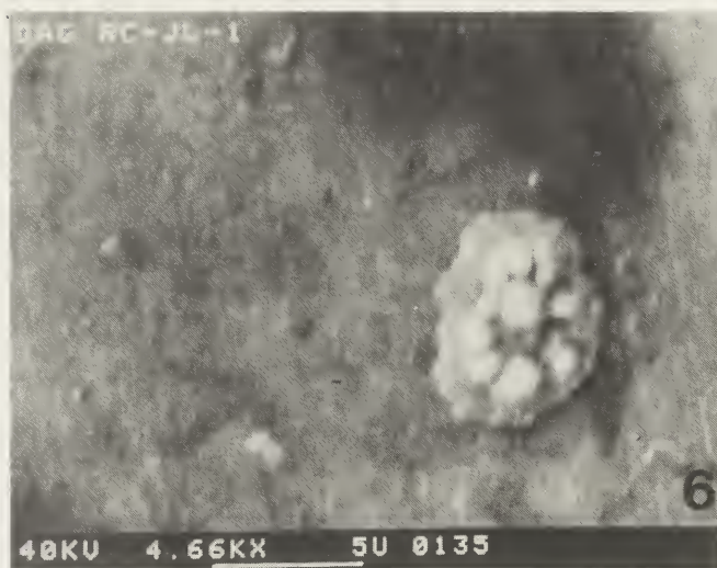
Figure 6 is from the shadow area of an uncleaned daguerreotype. The diffuse etching seen as the darker overall patterning on the plate surface is from droplets of highly alkaline solutions, probably sodium hydroxide with dissolved silicates, which fall from the cover glasses. This etching is not found uniformly distributed over the plate. Further, it is clearly not related to the more severe damage caused by solvent cleaners. It should be noted that only a very small number of nineteenth century daguerreotypes have never been cleaned. Thus, this diffuse etching is not often observed. The scale bar is equal to 5 \mu m.
