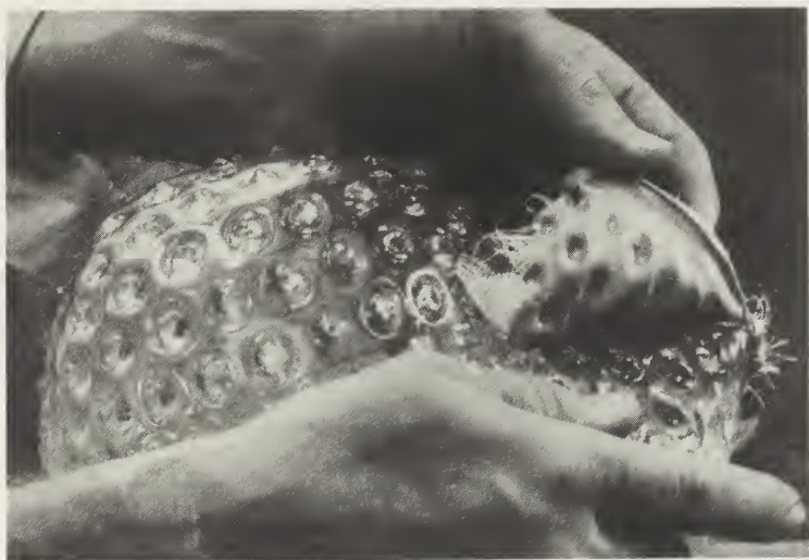
Photo 2/ Addition-type silicone rubbers are easily detached from surfaces which condensation-type rubbers would get stuck to
