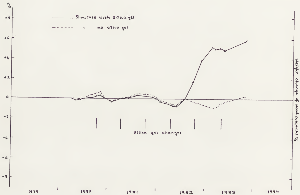
Figure 2. Weight loss of wood "object" in experimental showcases in laboratory with and without silica gel.
