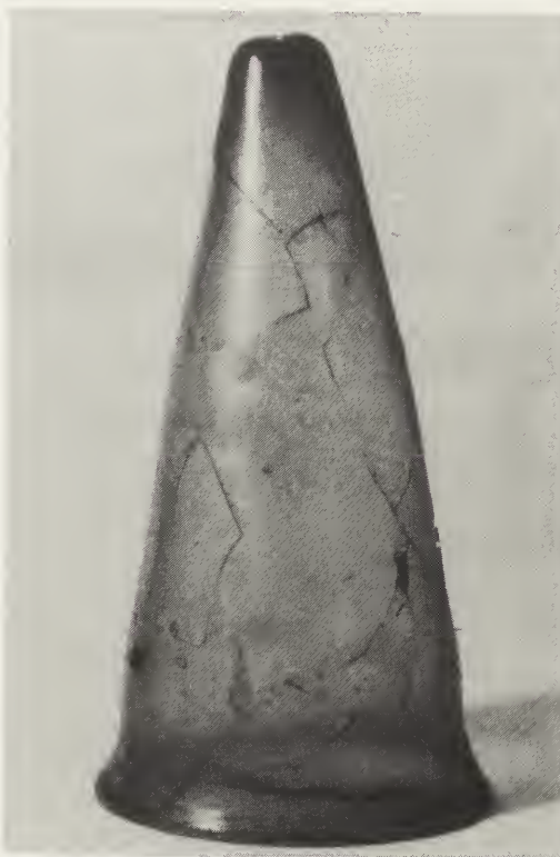
Polyester clear embedding resin (coloured with polyester pigments) has been poured between the two wax sheets and allowed to cure in situ . The wax sheets are then removed.
