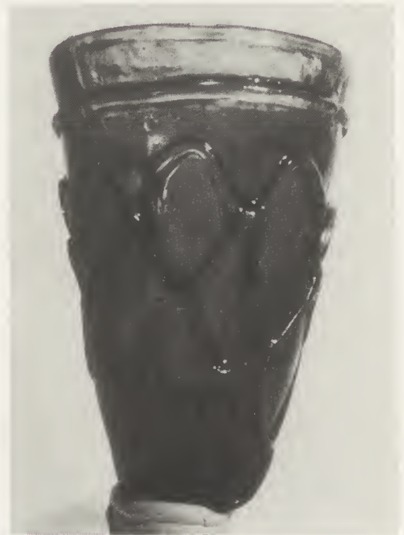
The Aloplast is removed, the mould replaced and filled with polyester clear embedding resin (coloured with polyester pigments).
