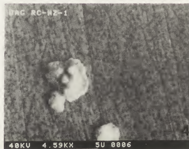
Figure 4 shows a shadow area of a daguerreotype cleaned with a thiourea cleaner. Even though the scale is different, it can be seen that the overall etching and image particle dissolution is less severe than that seen in Fig. 3. The scale bar is equal to 5 \mu\text{m} .
