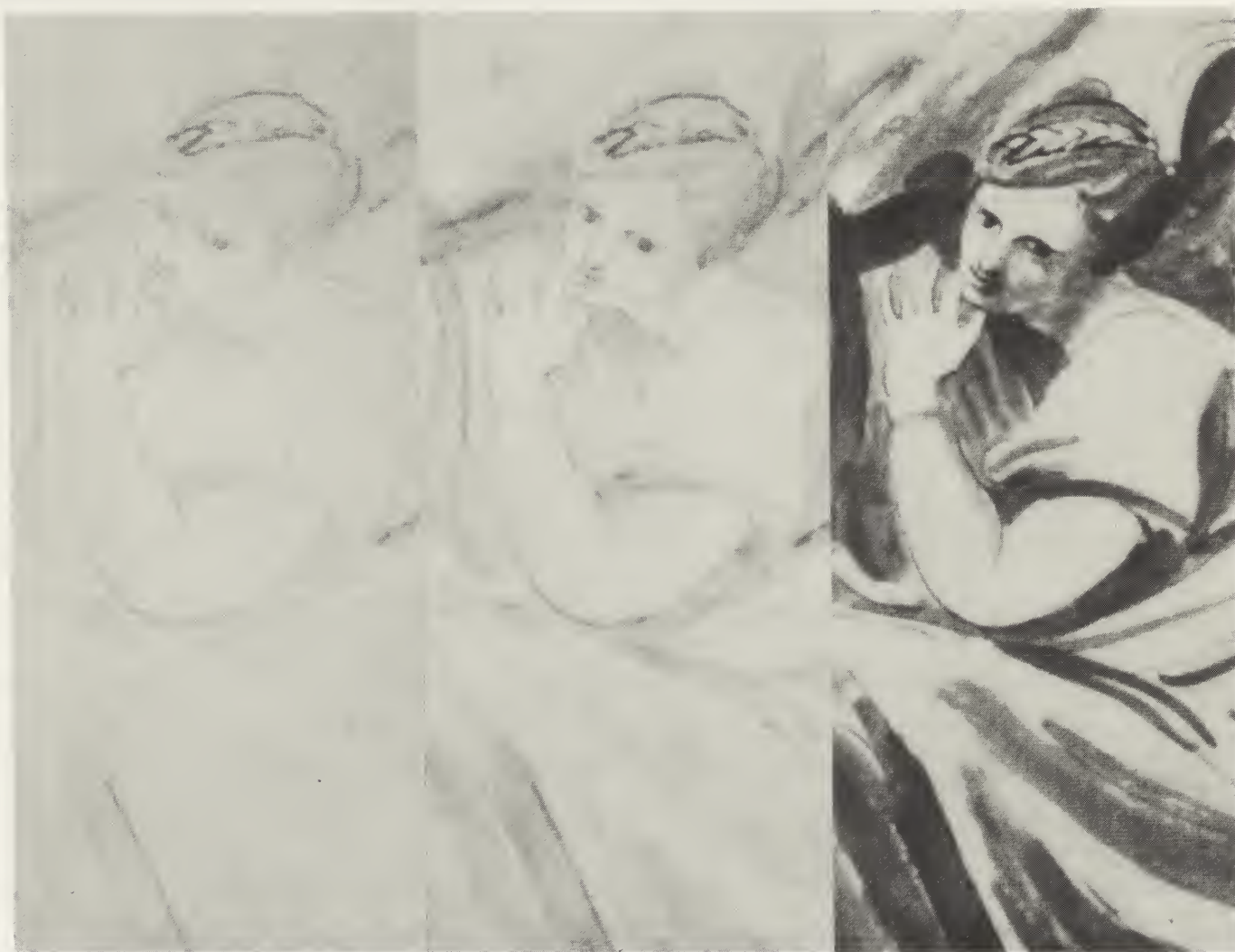
The three reflectograms above show the effects (from left to right) of Kodak filter 87A, 87C and no filter on a detail of a drawing by George Romney, Lady with a Lyre .
