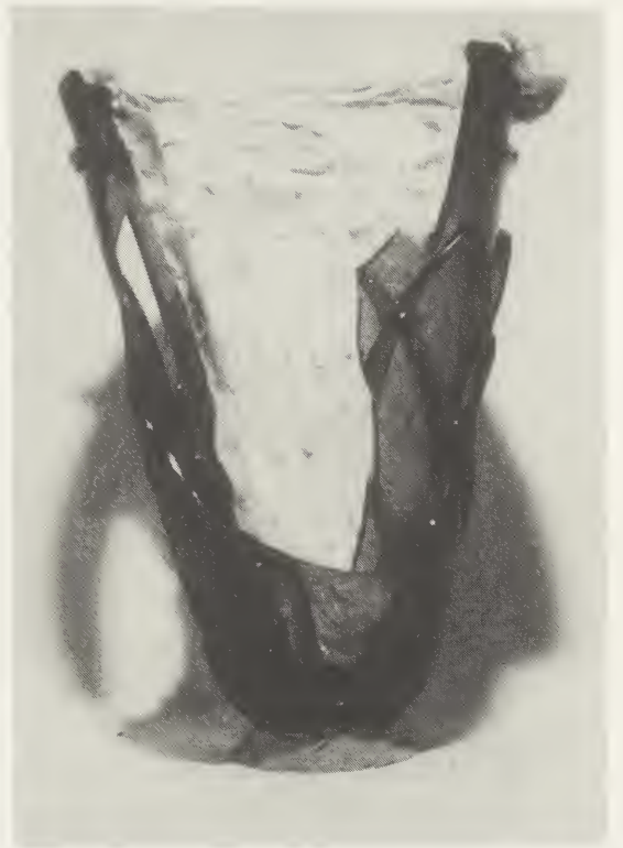
The rubber mould is re-located behind the missing area, a model of Aloplast is made to represent the glass. More silicone is then used to enclose the Aloplast.
