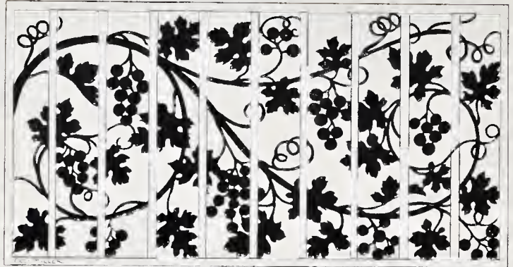
No. 7.—Design founded on the Grape. The uprights could form a sort of grille and be independent of the fret, or glued at the back of the fret to strengthen it.
