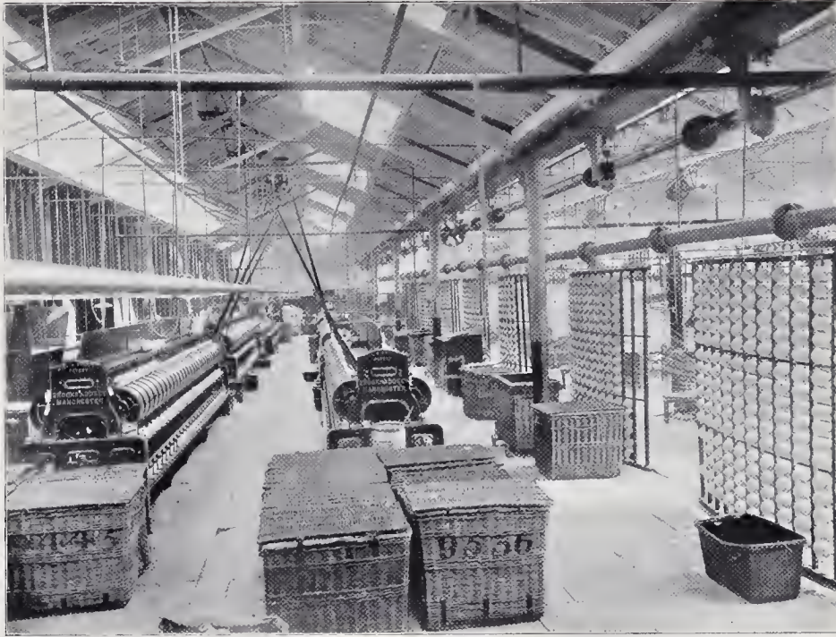
View of the Room in which the winding and warping of the Yarn is carried on.
