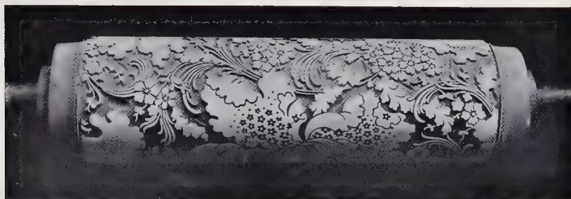
No. 1.—Engraved Roller for wall-paper printing: ground of wood, design in copper wire, outline filled in with felt.
