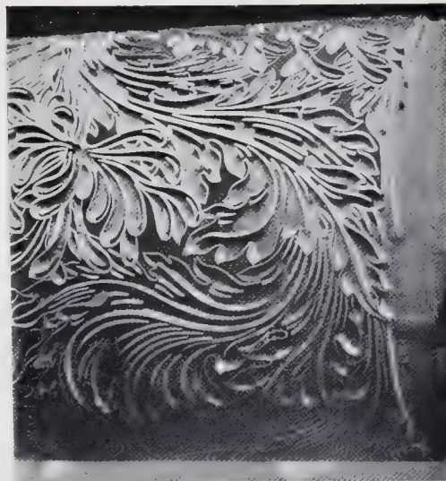
No. 4.—Detail of a Roller in raised metal outline upon wood.
