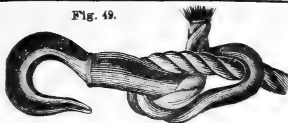
Fig. 49. SWIVEL ROPE HITCH.
