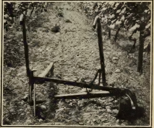
FIG. 200. The grape hoe may be thrown toward or away from the vines quickly by manipulating the left handle. The shovel on the right may be reversed to throw the soil toward the vines. A spring-tooth attachment between the disk and the shovel is also available.
