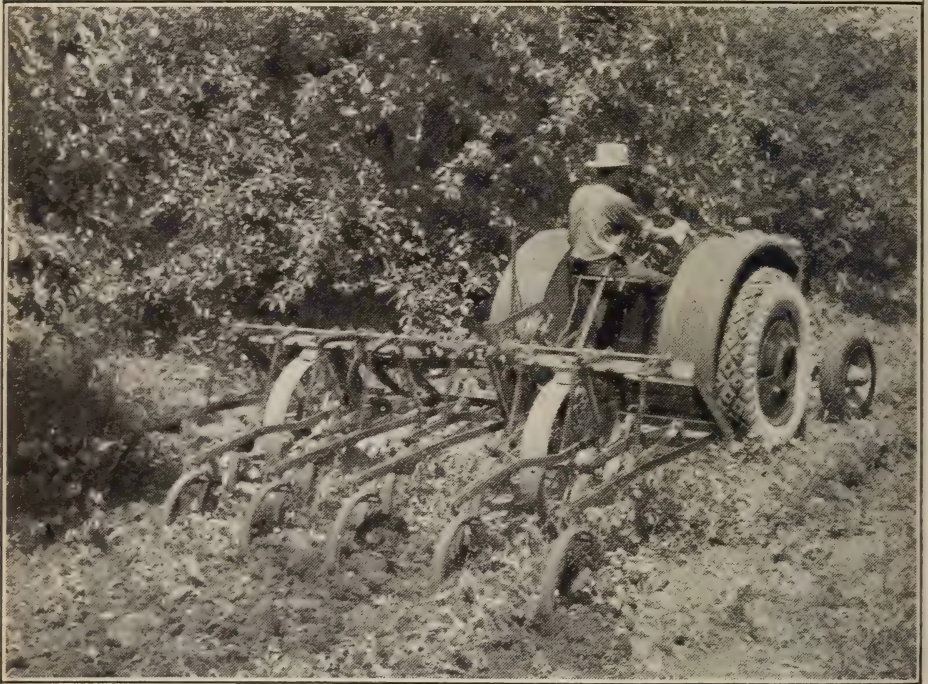
FIG. 169. This light-draft harrow is a very effective implement on land free from large stones or rock ledges.
