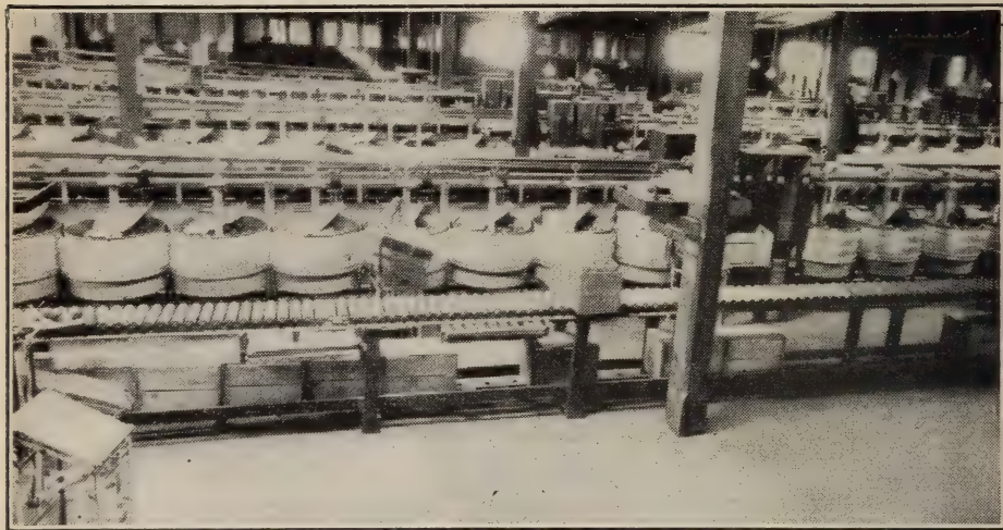
FIG. 14. A battery of rotary bin sizing machines, separating the apples according to weight. Each machine has forty-four bins, making possible eleven separations for size in several grades from the standpoint of quality. At the lower left are two stands mounted on castors. The packers place their boxes on them, wheel them from bin to bin, wrapping each apple and placing it carefully but rapidly in the box. In the immediate foreground is a conveyor, the top section taking the packed boxes away, the lower section bringing the empty boxes back. Boxes are stamped with variety and grade designations and with the number of apples in the box. Lidding presses fasten the covers. Each machine has a capacity of 200 packed boxes per hour.
