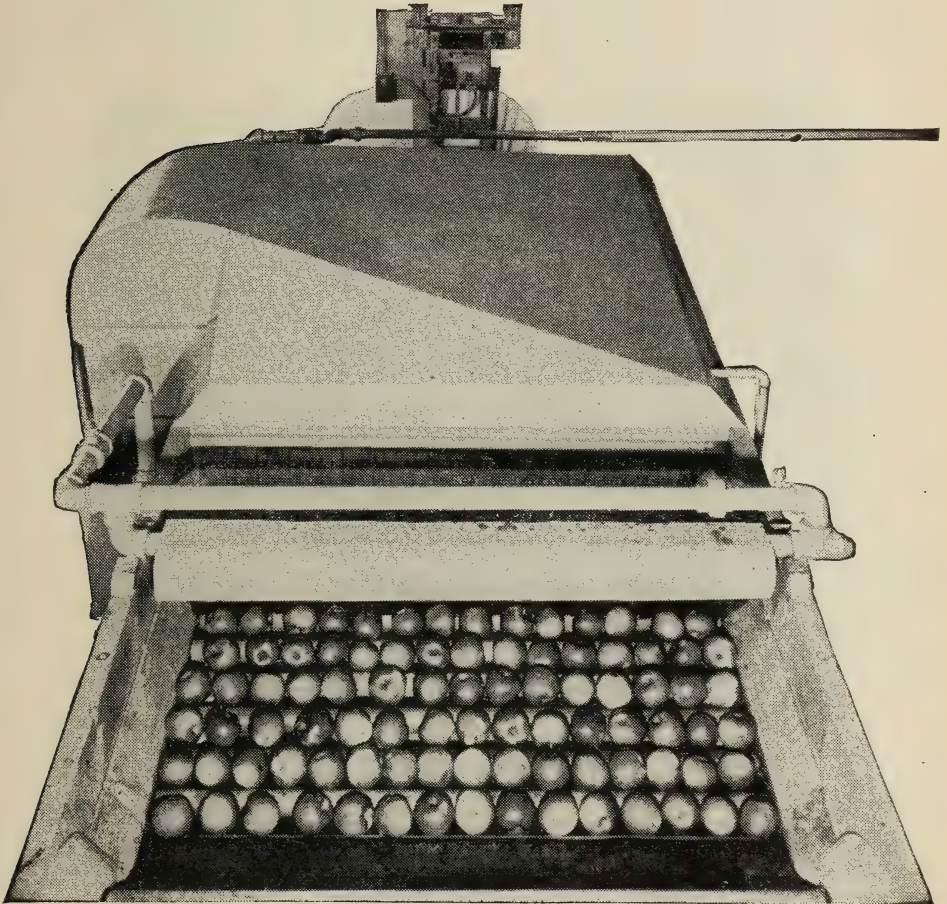
FIG. 28. A waxing outfit. The curved metal shield directs a sheet of wax over the revolving fruit. The machine has a capacity of 300 bushels per hour.
