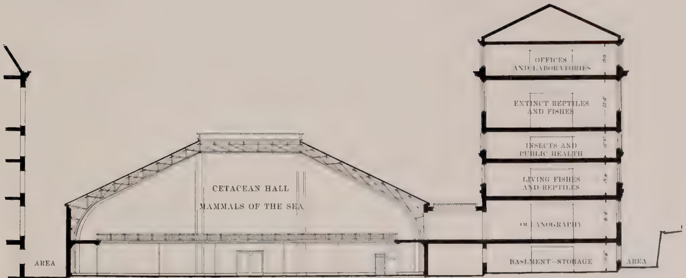
East and West Section through the Southeast Court, showing New Wing and Cetacean Hall
