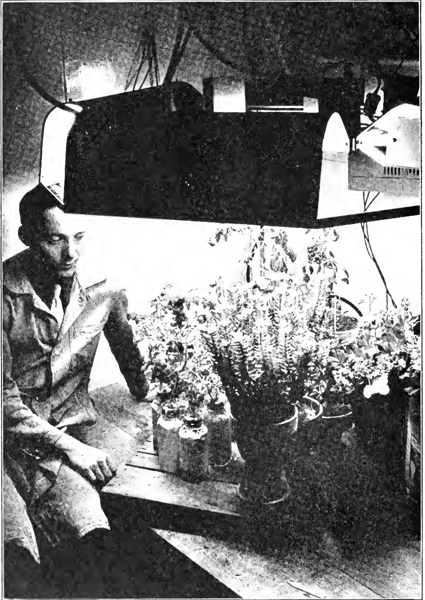
FIGURE 117. An arrangement of four 10,000-lumen sodium vapor lamps designed especially for plant work.
