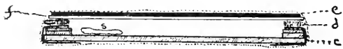
PLAN OF THE CROSS SECTION OF THE NEST. c, black cloth binding; d, Turkish toweling; e, cardboard cover; f, the dotted line represents the rubber band around the nest; s, sponge.
