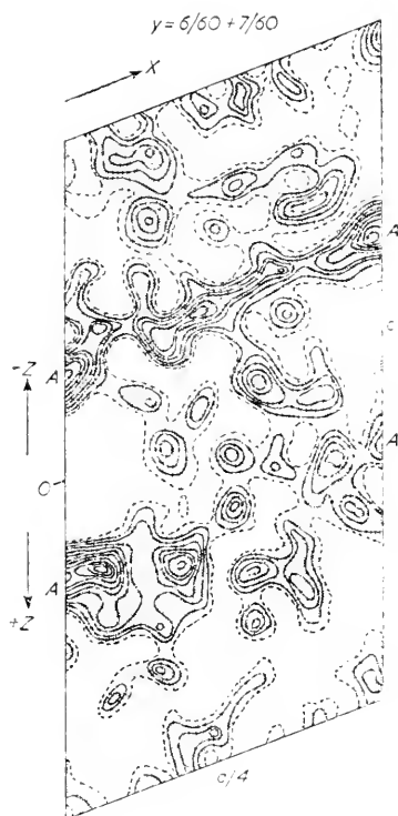
Figure 4. Contour map obtained by adding densities of sections 6.3 and 7.4 Å above the origin.
