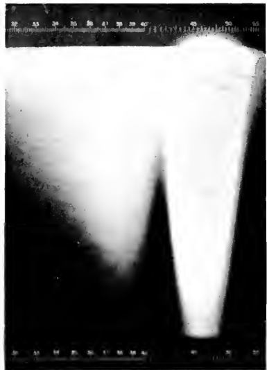
Figure 9. Spectrogram of a 35 per cent solution of HbO 2 in a 5μ layer, showing Soret band at 414.5 mμ but no band at 378 mμ.
