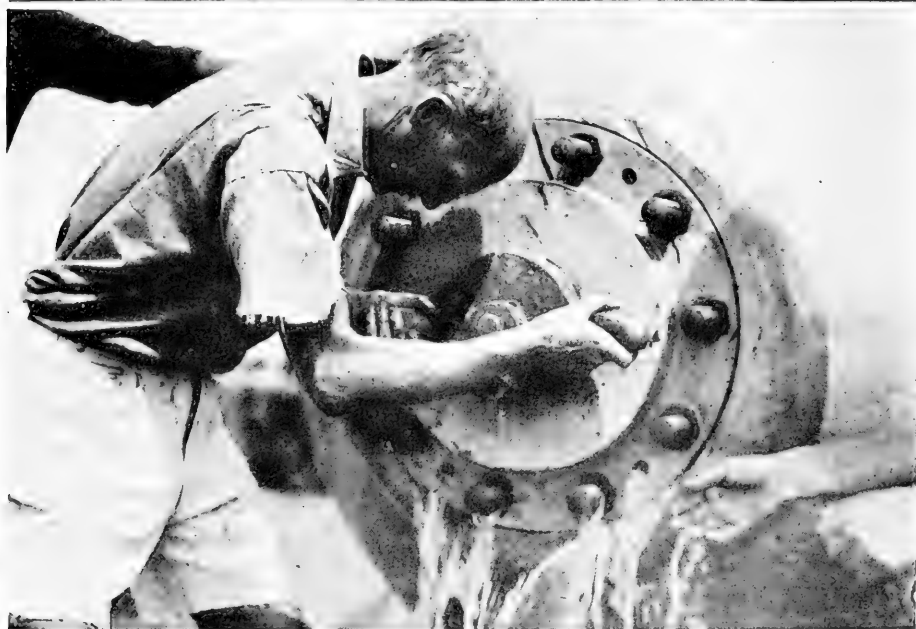
FIG. 73. ( upper ) The central wing-bolt is loosened and slowly turned, and almost at once water begins to drip out, the hissing increasing. FIG. 74. ( lower ) As the wing-bolt turns, more and more water escapes, and the hissing rises to a high scream. On the chance that the pressure might be dangerous, the deck is cleared of people, and the photographer placed far to one side.
