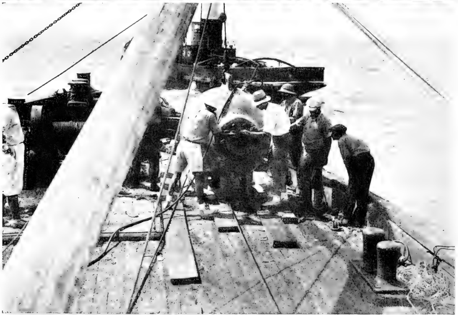
FIG. 71. ( upper ) Straining at its cable, the bathysphere swings heavily inboard and during a momentary lull between swells, is brought to rest on the landing boards. A glance at the new quartz window shows that a leak has started (see photograph) and that the sphere is filled with water—not from an explosion, but from an implosion. FIG. 72. ( lower ) For the first time in our work with the bathysphere something has gone wrong. The steel sides are cold, and a low hissing sound can be heard. Those near the bathysphere are Beebe, Tee-Van, Barton, Blagdon, and our favorite deck-hand known as OKay.
