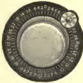
Fig. 54.—Risley rotary prism.
