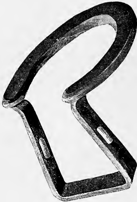
FIG. 395.—Patten hind shoe. Made from \frac{3}{4} \times \frac{3}{8} inch iron.
