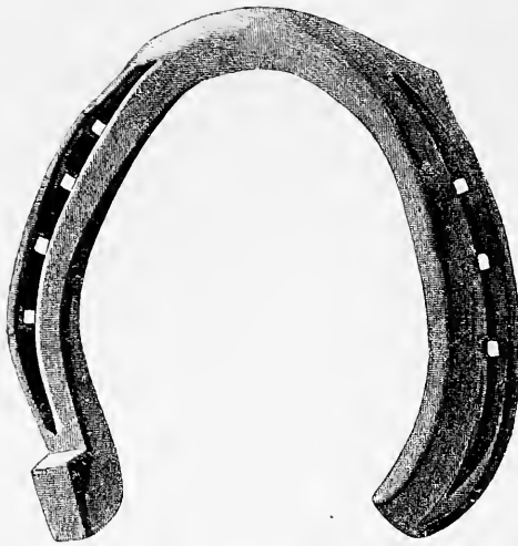
FIG. 290.--Fullered hind shoe, 'set' inside. Made from \frac{3}{4} square iron.
