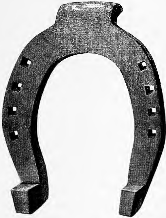
FIG. 328.—Stamped cart hind shoe, with toe-piece. Made from 1\frac{1}{4} \times \frac{5}{8} inch iron.
