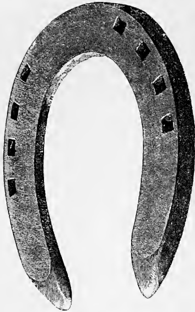
FIG. 253.—Stamped fore shoe (for railway shunting horses). Made from 1\frac{1}{2} \times \frac{5}{8} inch iron.
