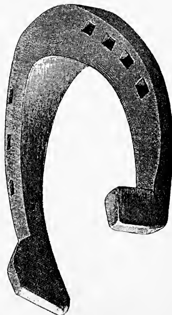
FIG. 244.—Stamped hind shoe (for omnibus work), with calkin and wedge heel. Made from old shoes.
