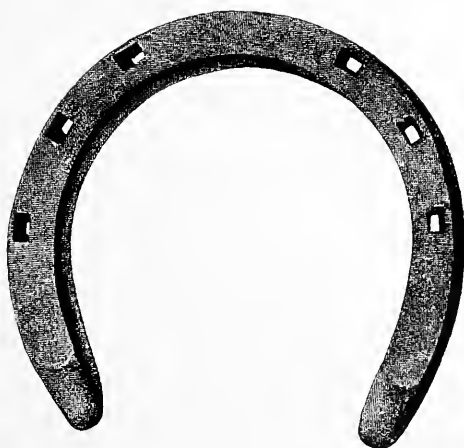
FIG. 219. Stamped fore shoe. Made from Charlier steel \frac{7}{8} inch square.
