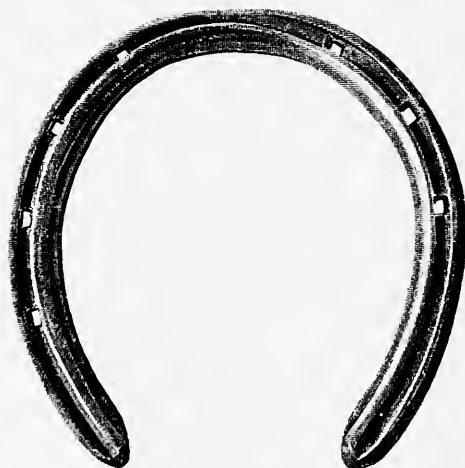
FIG. 227.—Concave fullered fore shoe for steeplechasing. Made from \frac{5}{8} \times \frac{3}{8} inch iron.
