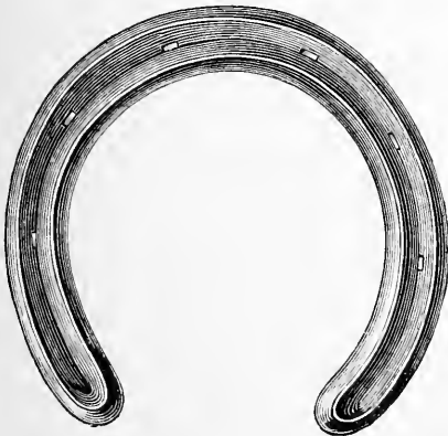
FIG. 111.—Count von Einsiedel's winter shoe for front feet.
