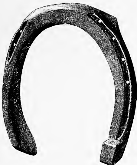
FIG. 288.—Partially feather-edged fullered hind shoe. Made from \frac{3}{4} \times \frac{1}{2} inch iron.
