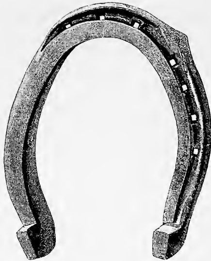
FIG. 286. - Fuller-edged feather-edged hind shoe (with two calkins). Made from \frac{3}{4} \times \frac{1}{2} inch iron.
