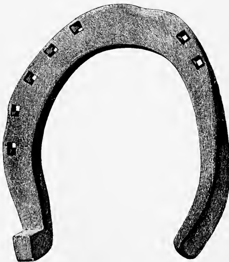
FIG. 287. - Feather-edged stamped hind shoe (with two nails inside toe). Made from \frac{3}{4} \times \frac{1}{2} inch iron.
