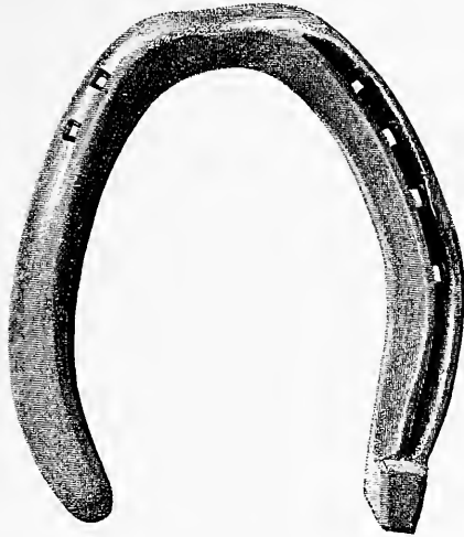
FIG. 222.—Concave partially-fullered hind shoe, made in concave tool, from \frac{3}{4} \times \frac{1}{2} inch iron, or from old shoes.
