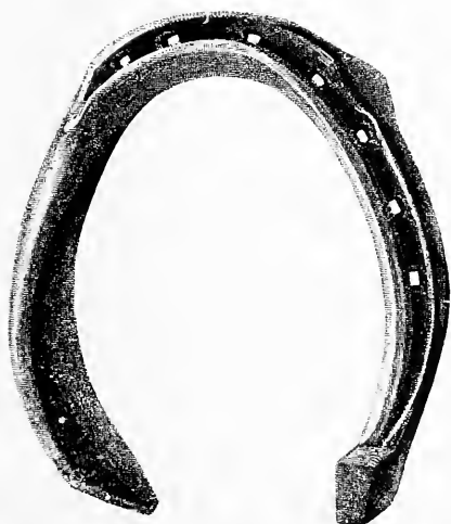
FIG. 297.—Concave partially-fullered feather-edged hind shoe. Made in concave tool from old shoes or from \frac{3}{4} \times \frac{1}{2} inch iron.
