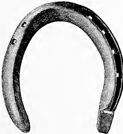
FIG. 221.—Concave partially-fullered hind shoe. Made of \frac{3}{4} \times \frac{1}{2} inch iron in concave tool.
