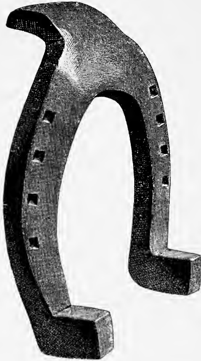
FIG. 246.—Cart horse hind shoe for town work, Made from old shoes.
