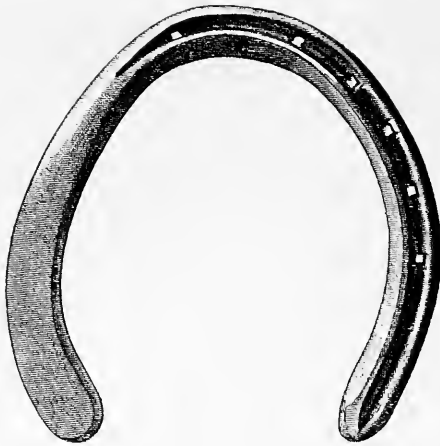
FIG. 298.—Feather-edged fullered concave fore shoe. Made in concave tool from \frac{1}{2} \times \frac{1}{4} inch iron or steel.
