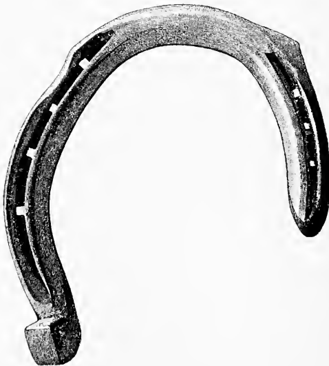
FIG. 299.—Concave three-quarter hind shoe. Made in concave tool from \frac{3}{4} \times \frac{1}{2} inch iron.
