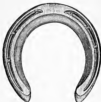
FIG. 274.—Right fore shoe with rounded inner edge (forging shoe).
