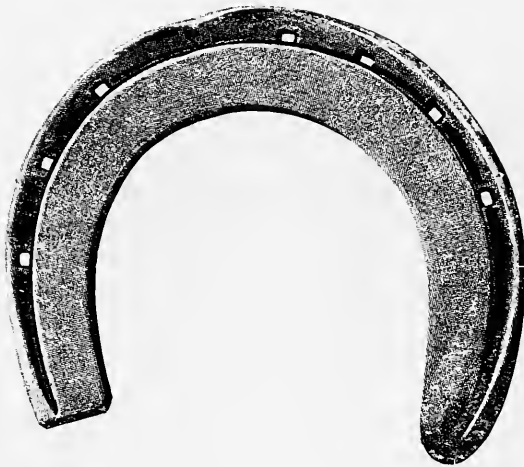
FIG. 370.—Three-quarter filled seated fore shoe. Made from 1 \times \frac{1}{2} inch iron.
