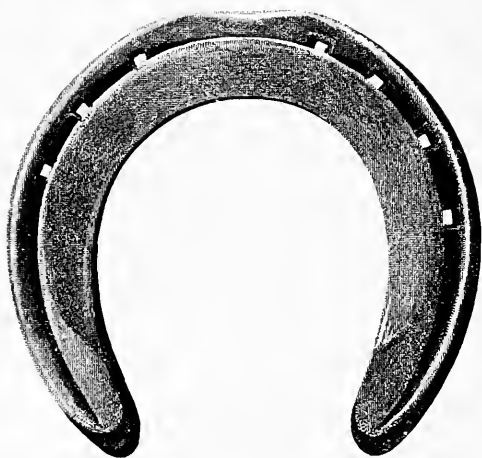
FIG. 242.—Fullered fore shoe (dished on ground surface). Made from 1 \times \frac{1}{2} inch iron.
