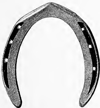
FIG. 277.—Diamond-toed fullered hind shoe (for harness horse). Made from \frac{3}{4} \times \frac{1}{2} inch iron.
