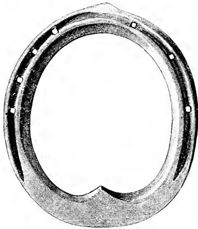
FIG. 314. —Concave bar fore shoe. Made in concave tool from \frac{3}{8} \times \frac{3}{8} inch iron.
