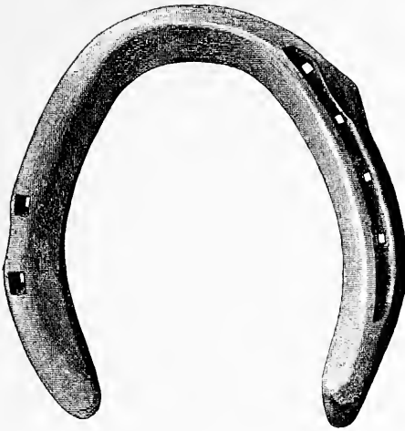
FIG. 220.—Concave partially-fullered hind shoe. Made in concave tool from \frac{3}{4} \times \frac{1}{2} inch iron or (preferably) from old shoes.
