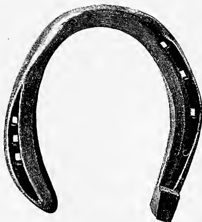
FIG. 295.—Fullered hind shoe for hack. Made from \frac{5}{8} \times \frac{1}{2} inch iron.
