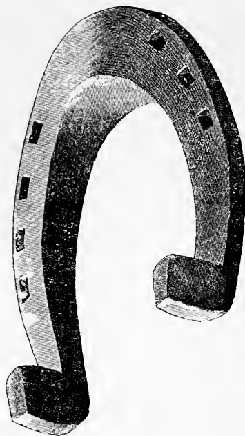
FIG. 243.—Stamped hind shoe (for omnibus work), with two calkins. Made from old shoes.
