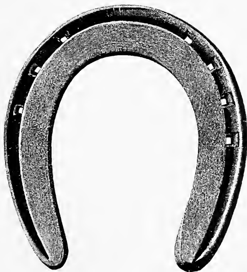
FIG. 241.—Thin heeled fullered seated fore shoe. Made from 1 \times \frac{5}{8} inch iron.
