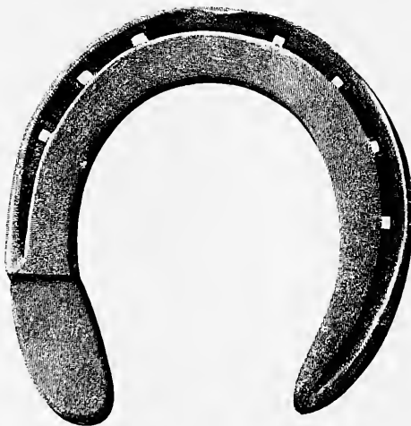
FIG. 371.—Fullered fore shoe ('set' on ground surface of inside heel). Made from \frac{7}{8} \times \frac{1}{2} inch iron.
