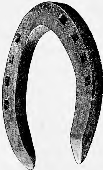
FIG. 254. — Stamped hind shoe (for railway shunting horses). Made from 1\frac{1}{2} \times \frac{5}{8} inch iron.
