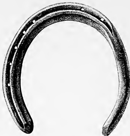
FIG. 294.—Fullered feather-edged concave fore shoe. Made from \frac{5}{8} \times \frac{3}{8} inch iron.
