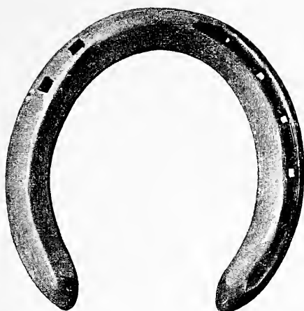
FIG. 218.—Concave fullered, feather-edged fore shoe. Made of \frac{3}{4} \times \frac{1}{2} inch iron in concave tool.
