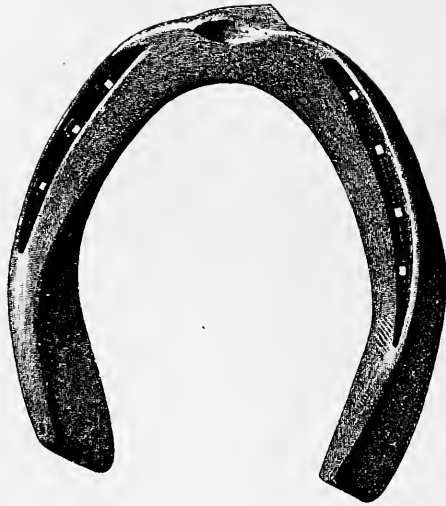
FIG. 391.—Fullered wedge-heeled hind shoe (for harness horse). Made from \frac{3}{4} \times \frac{1}{2} inch iron.
