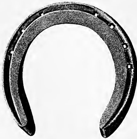
FIG. 211.—Fullered seated fore shoe with thick heels. Made of \frac{7}{8} × \frac{3}{4} inch iron.
