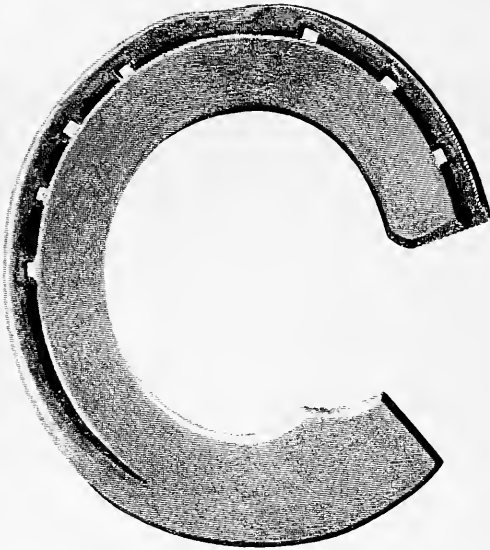
FIG. 318.—Fullered seated three-quarter bar fore shoe (for harness horse). Made from \frac{3}{4} \times \frac{1}{2} inch iron.
