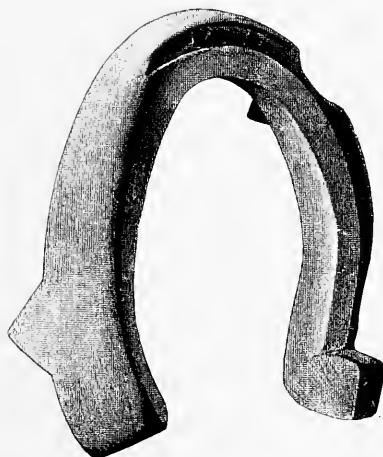
FIG. 289.—Partially-fullered feather-edged hind shoe. Made from \frac{3}{4} \times \frac{1}{2} inch iron.
