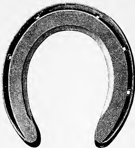
FIG. 216. - Fullered seated fore shoe. Made of \frac{3}{4} \times \frac{1}{2} inch iron.
