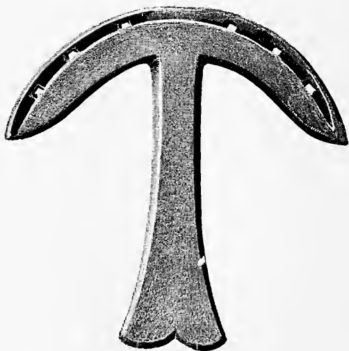
FIG. 338.—Tip for producing frog pressure. Made from \frac{3}{4} \times \frac{1}{2} inch iron.
