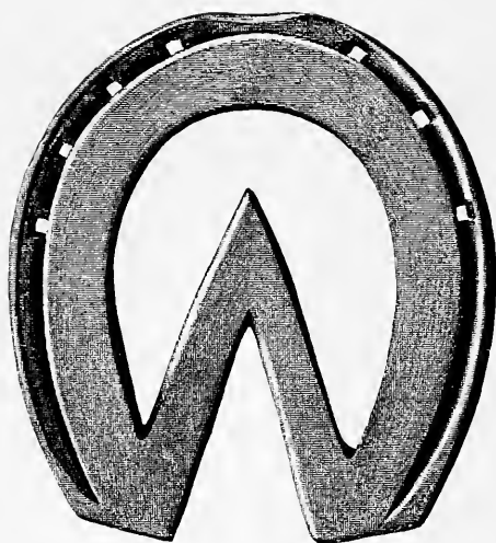
FIG. 337.—Fullered fore shoe (for harness horse), with frog plate. Made from 1 \times \frac{1}{2} inch iron.
