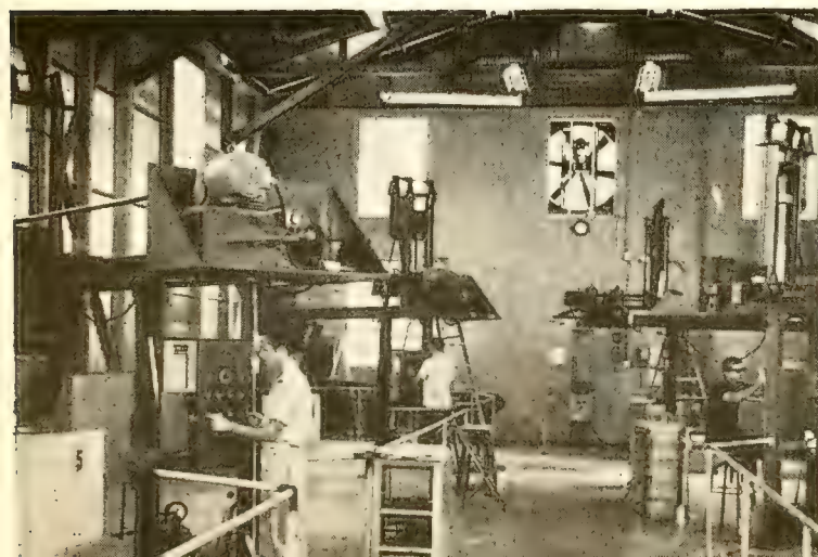
FIG. 3. COBALT ROOM HAS 6 IRRADIATORS, each of which performs 13-min irradiation automatically once operator has inserted canister and started operation
