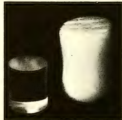
FIG. 12. After the slightly irradiated rod of polymethyl methacrylate (left) has been heated to about 120° C, it is expanded by bubble formation
