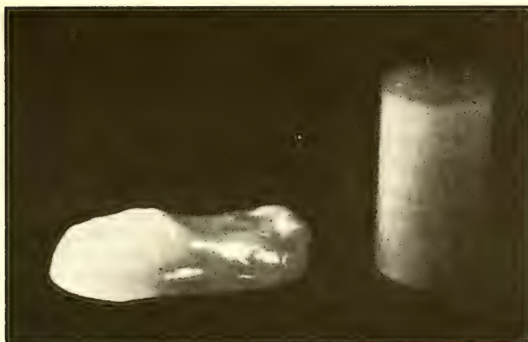
FIG. 1. Effect of irradiation on heat-resistant ( 120^{\circ}\text{C} ) properties of polyethylene. Control sample at left; shortly-irradiated sample at right
