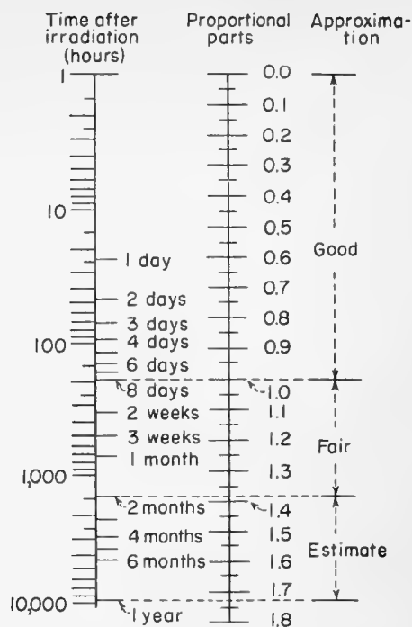
FIG. 9. Nomogram for estimating decrease in optical densities of glasses after different time intervals following irradiation and heating
