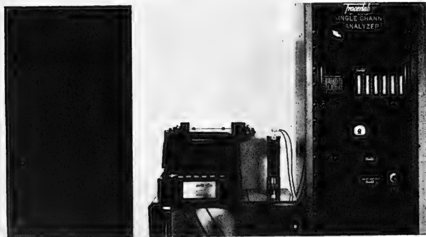
FIG. 3. Stepping single-channel analyzer offers automatic, unattended operation. Electric typewriter records window number, count, time, and time of day
