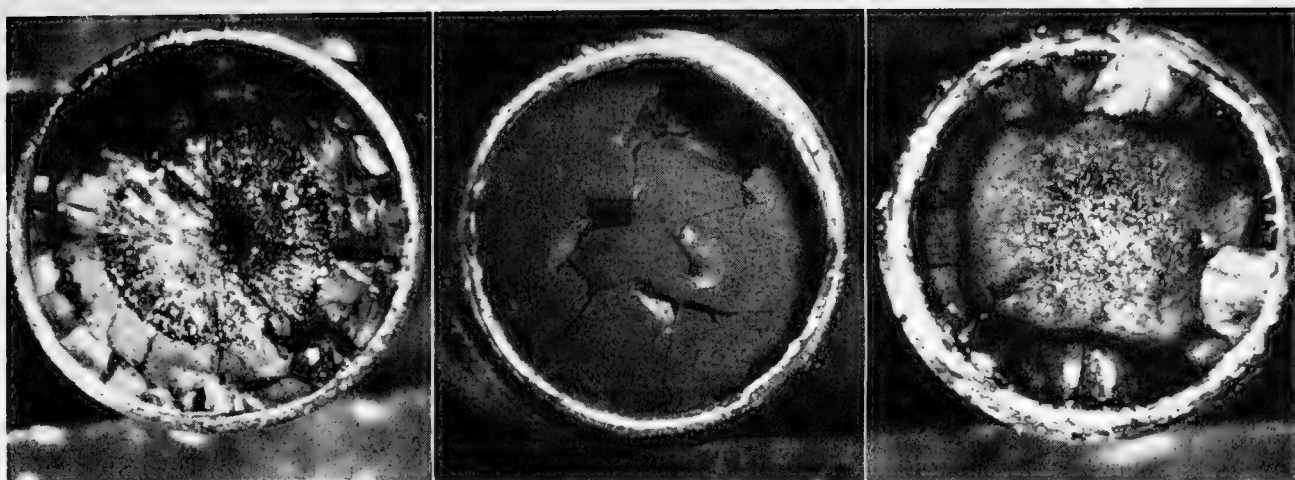
FIG. 7 Cross sections of irradiated Zircaloy-2-clad UO_2 rods. At left is 0.72-in.-diameter rod irradiated for 60 sec in NRX hydraulic rabbit; note central area that had been melted. Center
