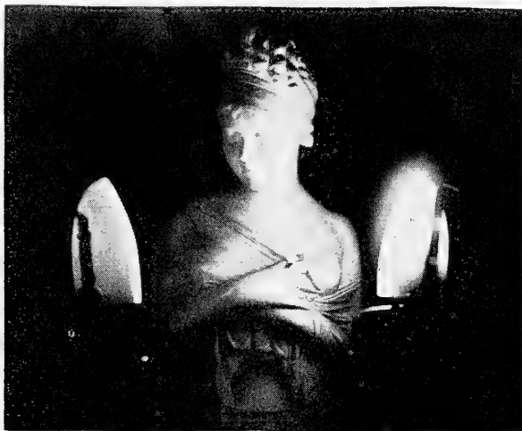
FIG. 5B.—Infrared photograph of the same subject made on infrared plates using heat of the flatirons as the only source of "illumination."
