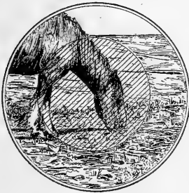
FIG. 12A.—Range finder in focused position.
