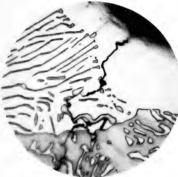
FIG. 15B.—Internal stress raiser in cast iron. This is the same as Fig. 15A but at a magnification of 3700 \times .
