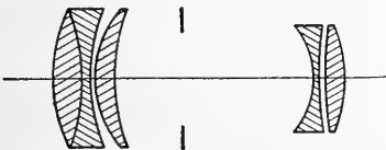
FIG. 56.—Taylor-Hobson 2.3\times , f/5 distortionless telephoto.
