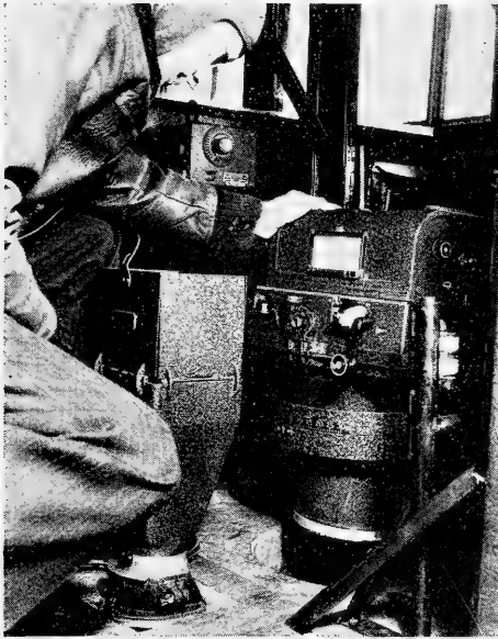
FIG. 15.—Standard single-lens camera installation. Photographer is looking into view finder above his hand. On the side of the cabin is the intervalometer for automatic camera operation.
